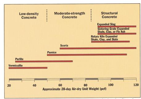
Don't confuse structural lightweight aggregate concrete with low-density and moderate-strength lightweight concretes.
