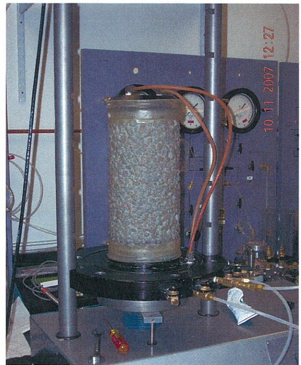
Photo 2 - Prepared lightweight aggregate test specimen under vacuum
