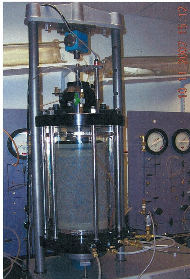
Photo 3 - Specimen in triaxial test cell apparatus prior to testing
