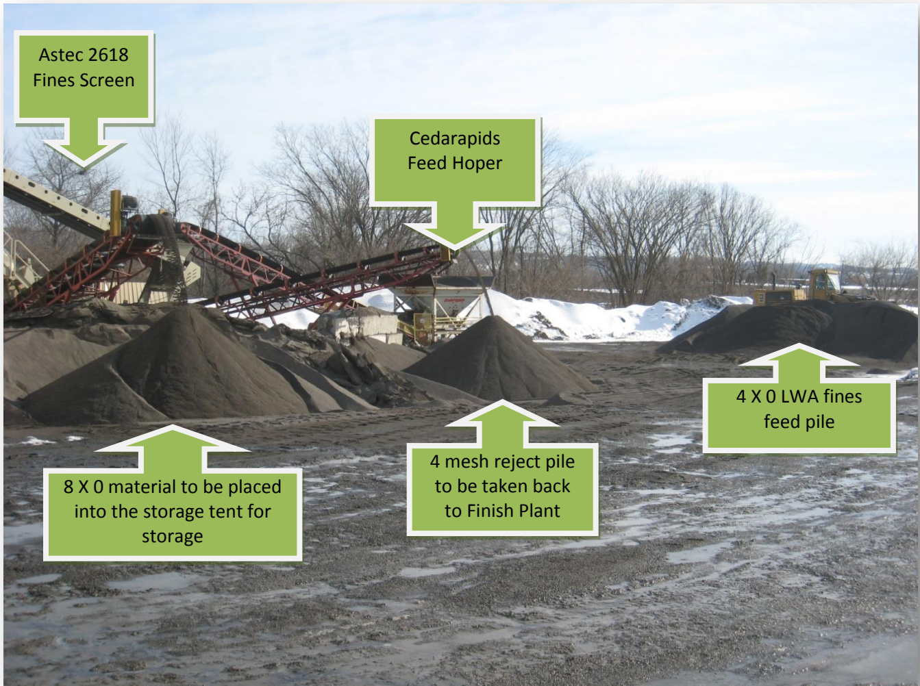
Figure 3. 4 X 0 LWA fines processing area. The 4 X 0 LWA fines are brought up from the Finish Plant and placed into a feed pile. The material is then fed into the screen feed hopper. A pile of 4 mesh reject material is created as well as a pile of 8 X 0 material which is placed inside the storage tent.
