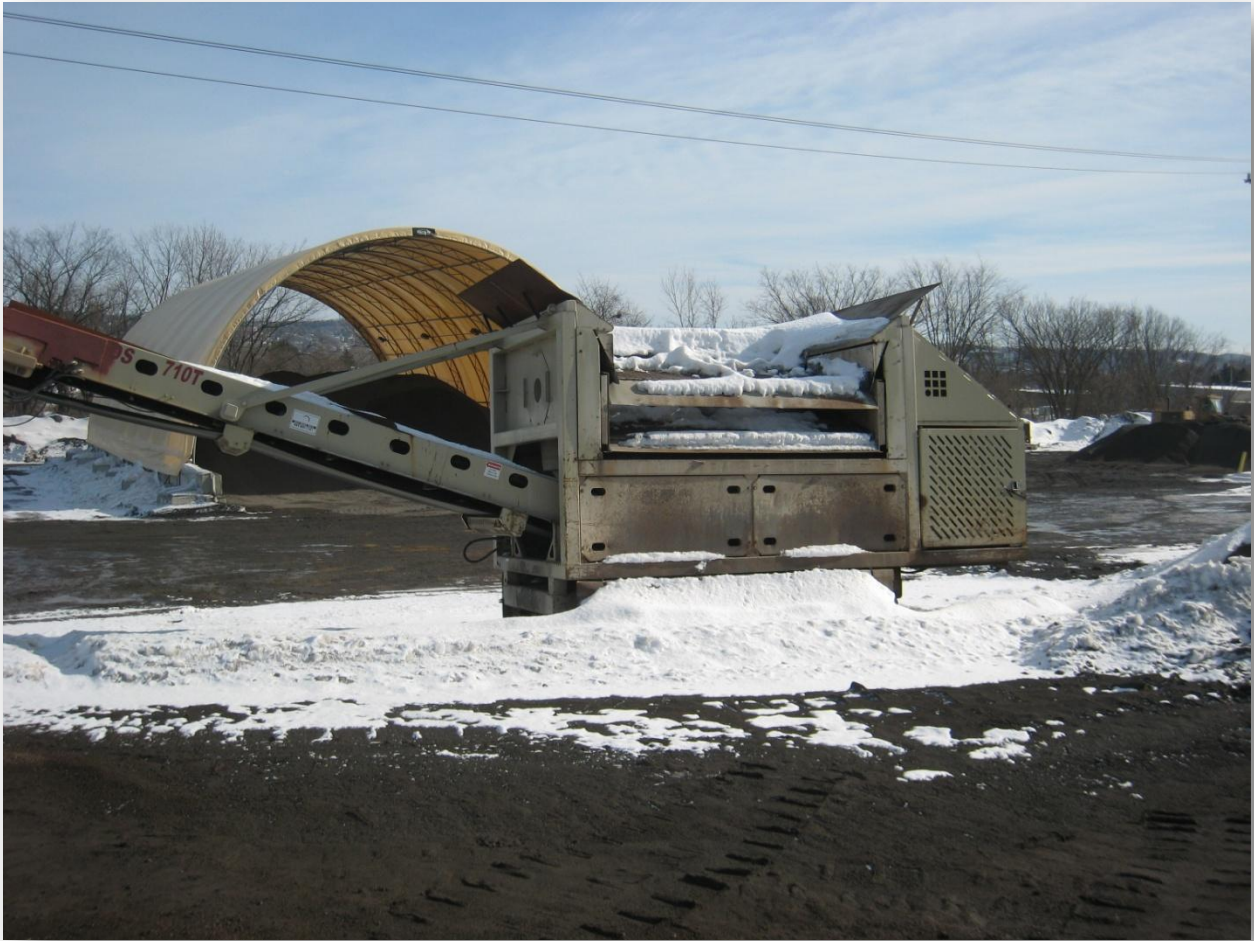
Figure 8. The Astec 710T screen is used to screen material from the long term block mix storage pile to remove clumped material or large frozen material. The Astec 710T and the Read screen can be used interchangeably.
