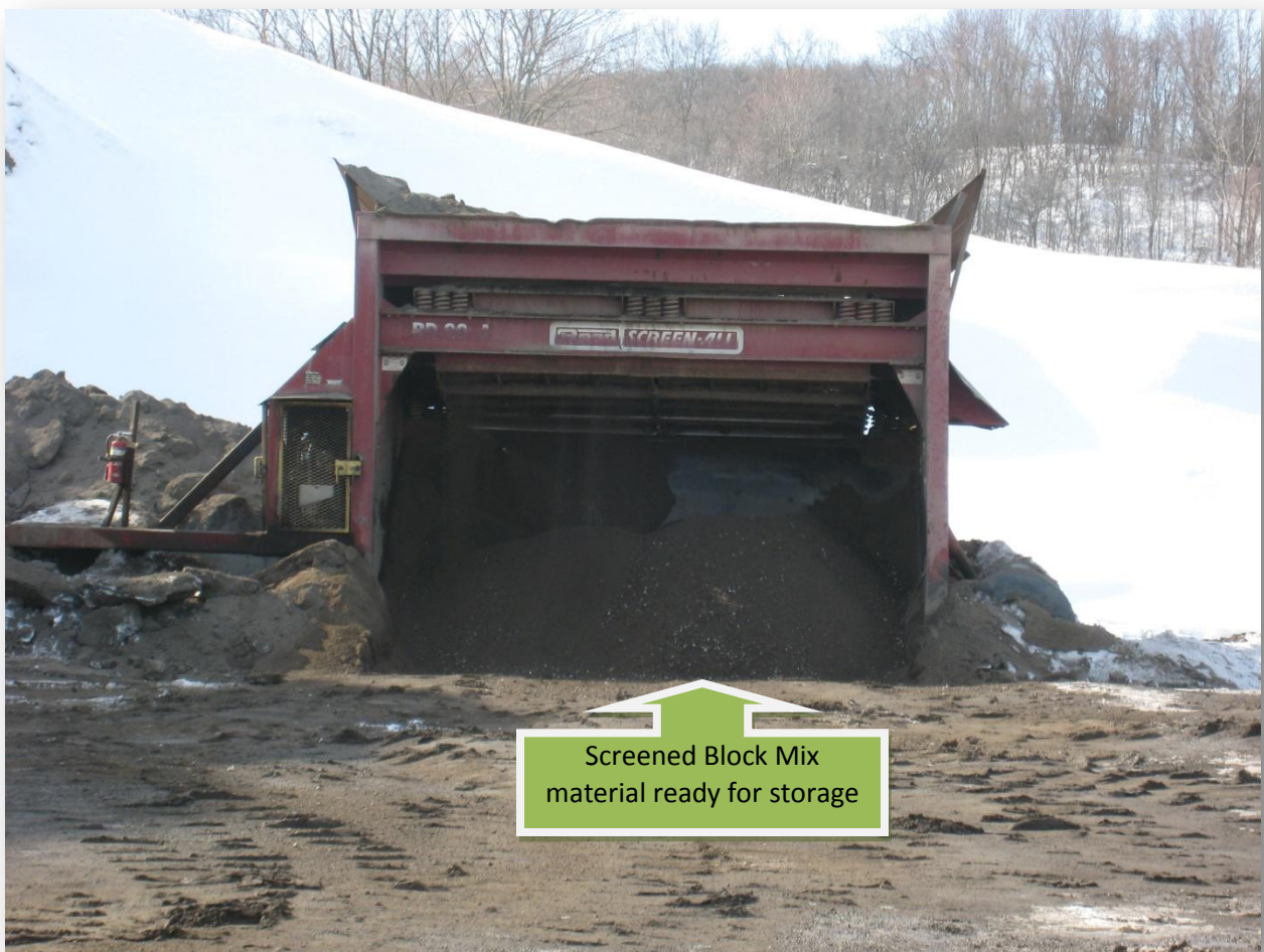
Figure 7. The Reade screen is used to screen material from the long term block mix storage pile to remove clumped material or large frozen material. The Reade screen and the Astec 710T can be used interchangeably.
