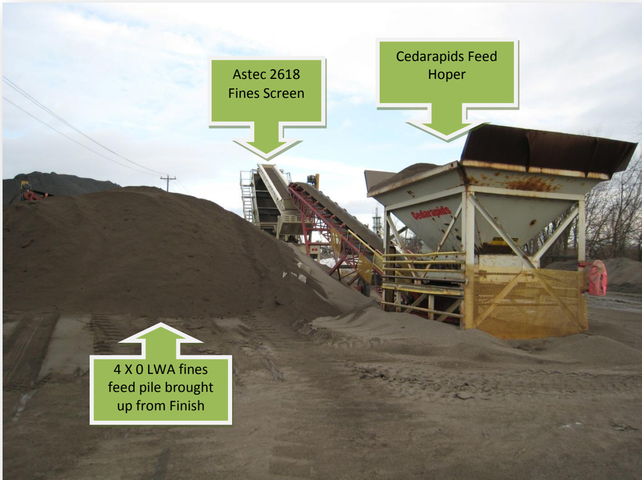
Figure 4. This is a close up photo of the Cedarapids Feed Hoper and the Astec 2618 Fines Screen used to process the 4 X 0 LWA fines.
