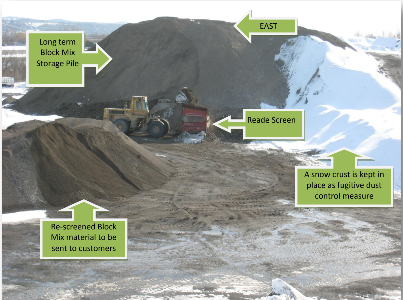
Figure 6. Block Mix Screening area. Block Mix is screened using either the Reade Screen or the Astec 710T to remove large chunk material. It should also be noted the working face of the long term storage pile is on the east side (leeward). The prevailing winds are out of the west and south.
